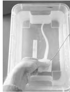
Figure 7. Physical coupling between a silicone appendix (cast onto a servo motor) and its containing medium (water). The arm produces fluid motion with gradual biomorphic bending when submerged in water but flaps clumsily around when in the air. Video: https://youtu.be/ifLChDLxdjE . ©Jonas Jørgensen
