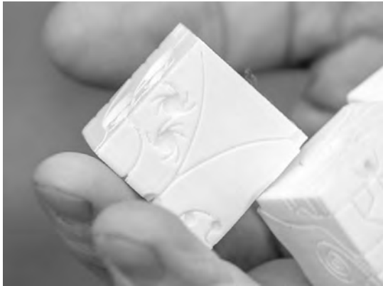
Figure 6. A Fluid Cube: example of Fluid Processor cubes that have been CAD constructed and 3D printed in corn starch based PLA. ©Stenslie 2016
