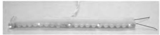
Figure 1. Caterpillar-inspired soft robot by Huai-Ti Lin, Gary G. Leisk and Barry Trimmer. ©Huai-Ti Lin, Gary G. Leisk and Barry Trimmer
