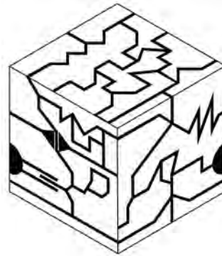
Figure 4. The Fluid Cube: layout of a cube-shaped Fluid Processor showing channels carved into solid material. ©Stenslie 2016
