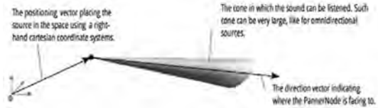
Figure 1. The PannerNode object takes multiple parameters. This project specifies a position while leaving the sound cone omnidirectional. Image by Mozilla Contributors is licensed under CC-BY-SA 2.5
