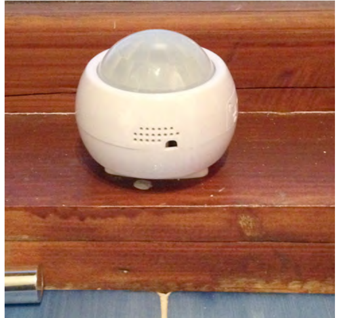
Fig. 4. Wireless passive infrared sensor installed in authors bathroom during pilot period. © Chris Speed.
