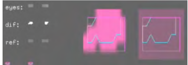
Fig. 4. Our custom blink detector. On the left the extracted eyes are drawn. On the right the detected blob is drawn, signaling the detection of a blink.
