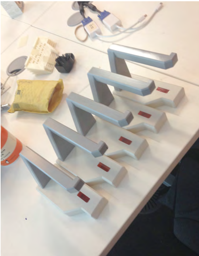
Fig.5. First batch of instrumented toilet roll holders prior to distribution. © Chris Speed.
